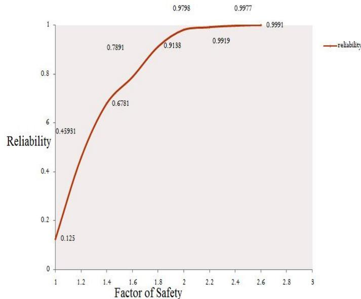
**Fig.1: Reliability of Gear pair system Vs factor of safety**
