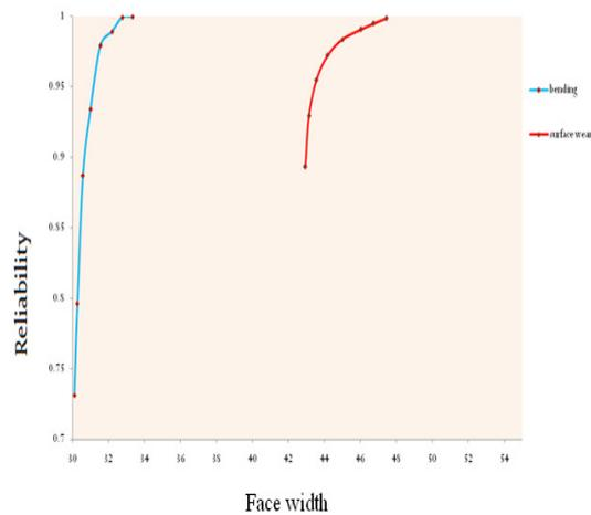
**Fig.2: Reliability of Gear pair system Vs face width of gear**
