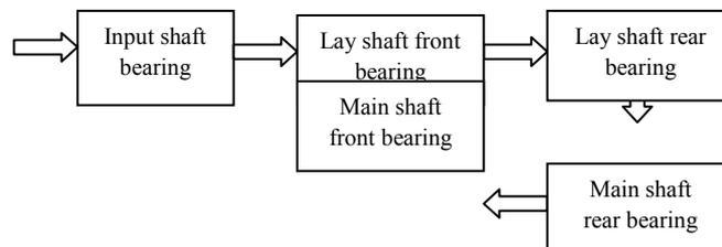
**Fig.6: Reliability Block Diagram of bearing system.**
